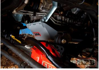
The engine/gearbox skid plate panel is attached to the existing gearbox cross-member at the rear and is supplied with a three piece cross-member for the front mount that attaches to the vehicles engine mounts.
